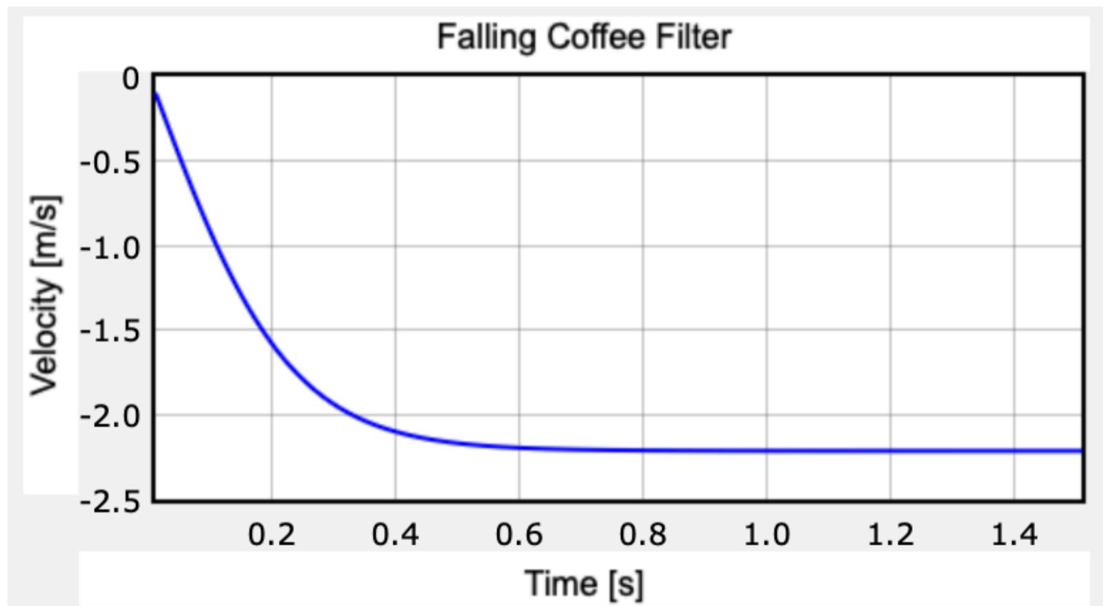
That's exactly what you would expect. You can see that horizontal line representing the terminal velocity of the filter.
