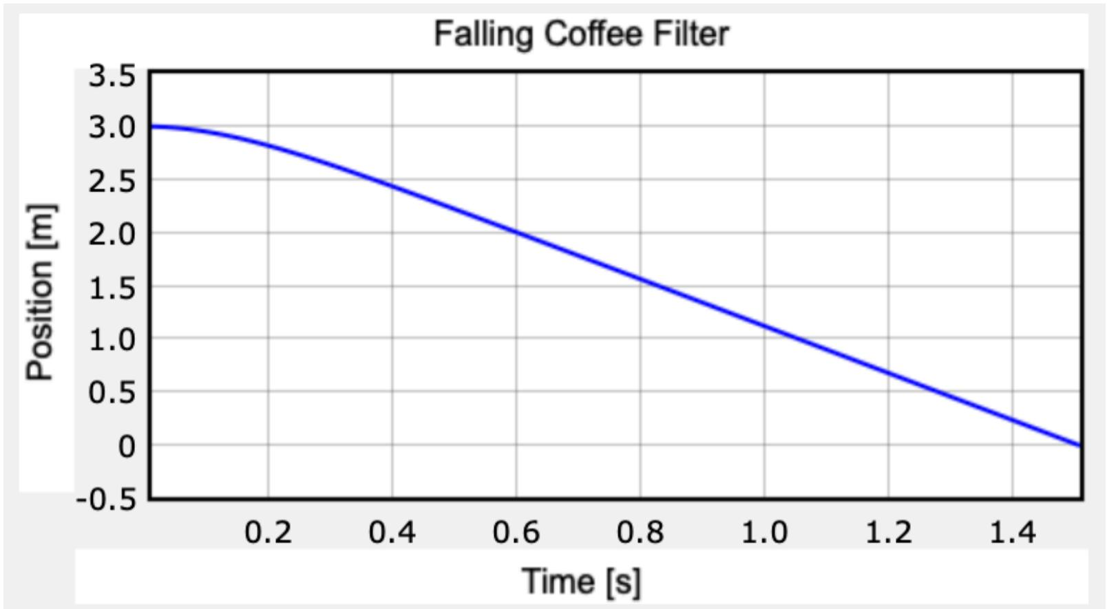
Notice that the coffee filter quickly reaches a terminal velocity. Just for fun, let's plot the velocity as a function time.
