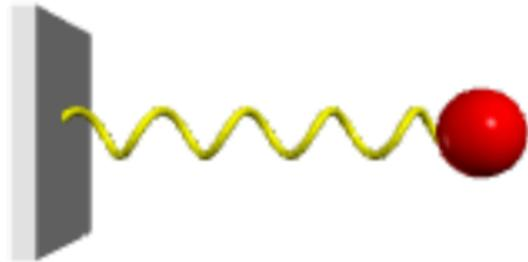
In this case, we can say that at the equilibrium position where the spring doesn't exert a force, the mass is at  $x = 0$  meters. As you pull the mass in the positive  $x$ -direction, the spring will pull back in the negative direction. We can write the force due to the spring as:
