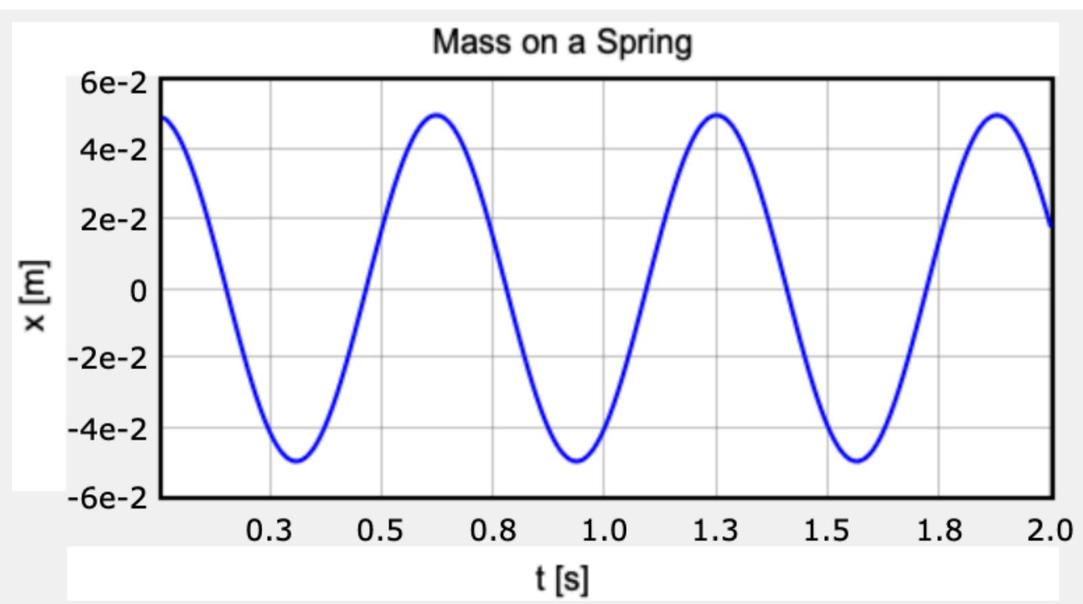
Why is this so awesome? It's because it's correct. Imagine that you started with Newton's second law and solved the equation of motion using your differential equation tricks. You would get the following function.
