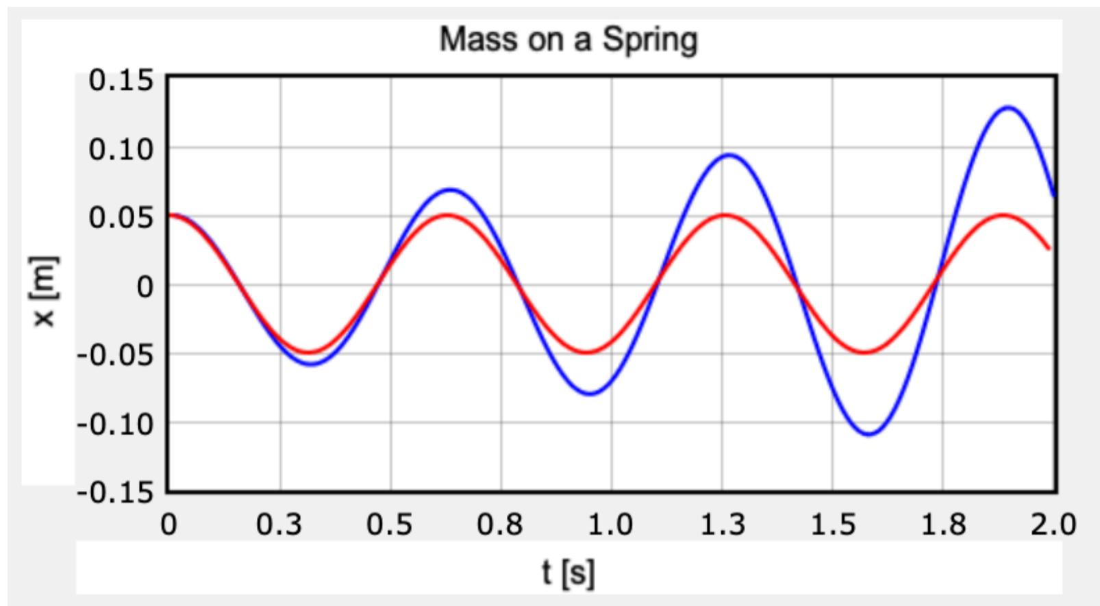
Yeah, that doesn't look right. The numerical model shows the amplitude of oscillation increasing as time increases. So, energy is not conserved. Can we fix this by using a smaller time interval? Sort of. Here's a time step of 0.001 seconds.
